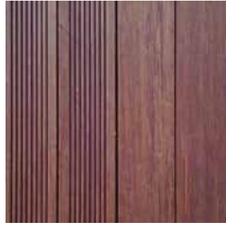
Surface of Bamboo X-treme with different maintenance and cleaning scenarios: weathered, dirty decking (left), weathered, cleaned decking (middle), and re-oiled decking (right).
