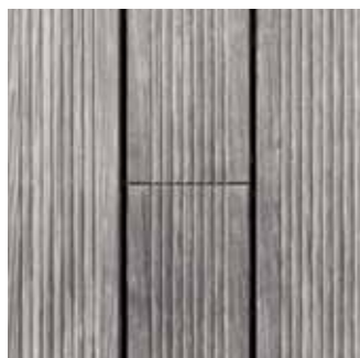
Gradation of greying of Bamboo X-treme over time: new, non-weathered decking (left), after 3 months of weathering (middle) and after 18 months of weathering (right).
